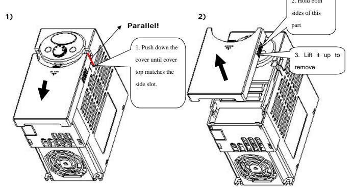
• Removal for wiring input power and terminals: After removing the front cover, lift the bottom cover up to disconnect.
